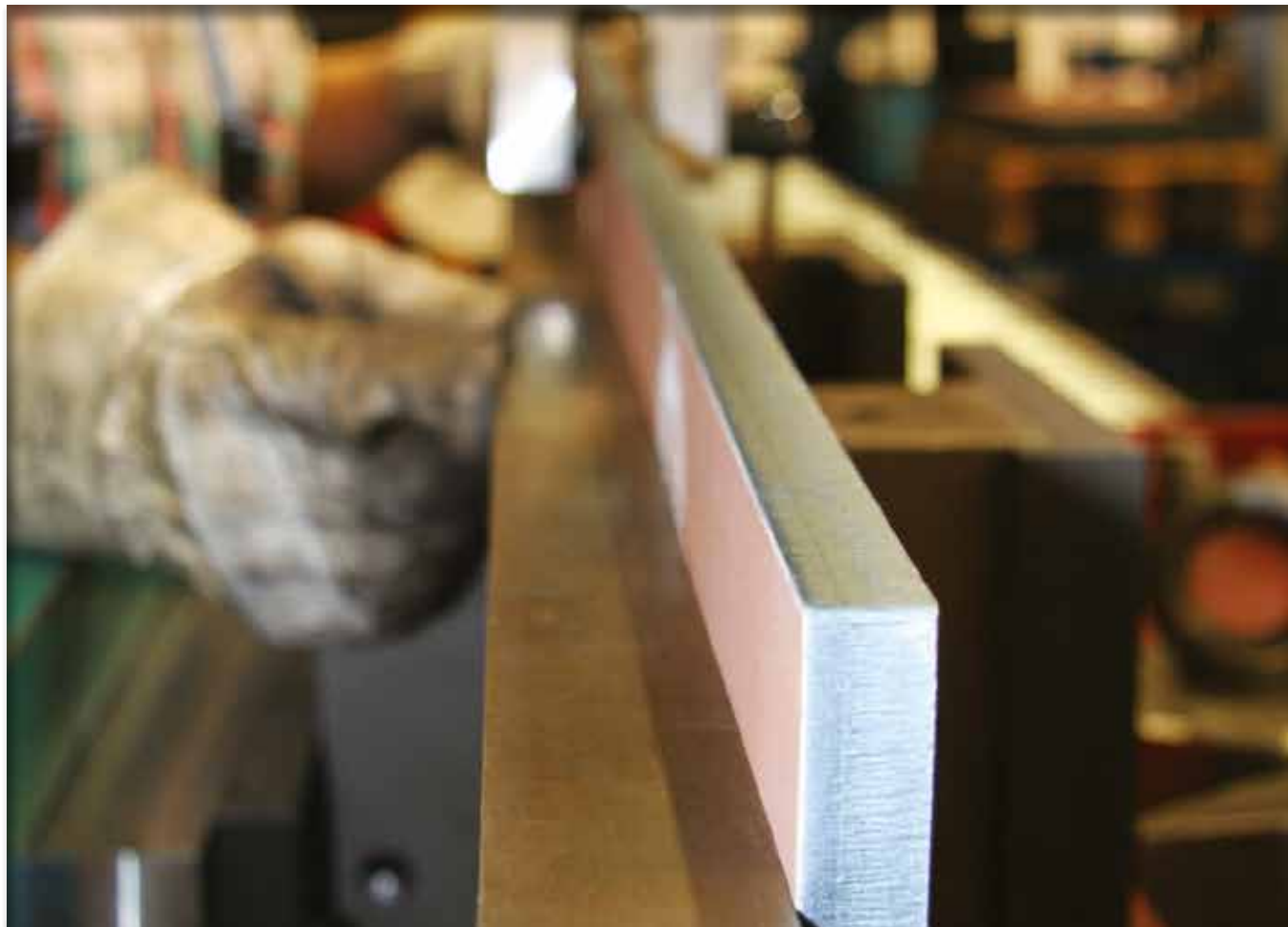
Tension-free alignment with an evenness error of max. 2/10 mm ensures a long service life, as the screed plate wears evenly.
