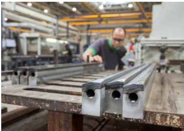
Tamper and pressure bar are hardened to a uniform depth of 5 mm.
